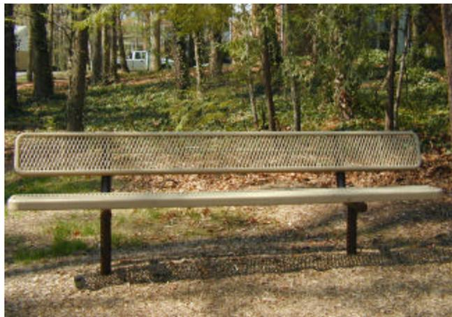
Benches are anchored in concrete and are constructed of steel and coated with molded PVC, or can be constructed of recycled plastic. A typical park bench is shown here.
