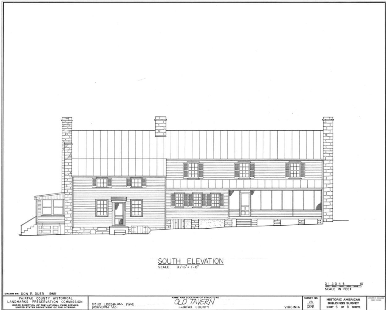
Figure 12. Dranesville Tavern south elevation HABS drawing, 1968. Note the screen at the south porch (Historic American Building Survey VA-503).
