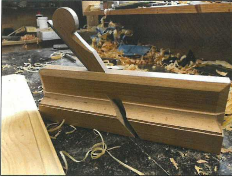
Building of wooden planes for running of moldings and sash parts.
