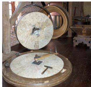
In the **mill**, students learn what types of resources aid the process of grinding grain into flour or cornmeal by the water-powered grinding stones.
