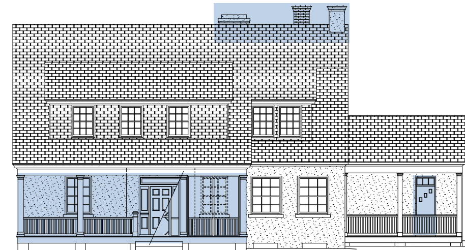
Figure 4.1 Areas shaded in blue are restoration areas. The stucco on the chimneys should be restored, the front porch screening should be removed, and a period-appropriate door, based on the house's existing door designs, should replace the current non-historic door. All non-shaded areas on this elevation will be preserved.
