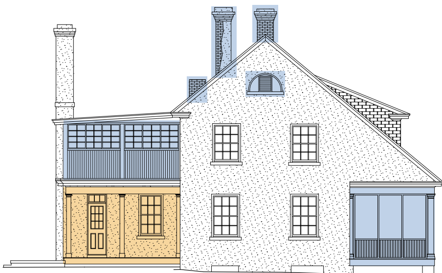
Figure 4.4 In addition to those areas shaded on the previous elevations, this elevation shows the attic lunette window shaded in blue. Restoration of this feature will include the replacement of the current rectangular vent and plywood with a louvered vent that fits the shape of the opening.
