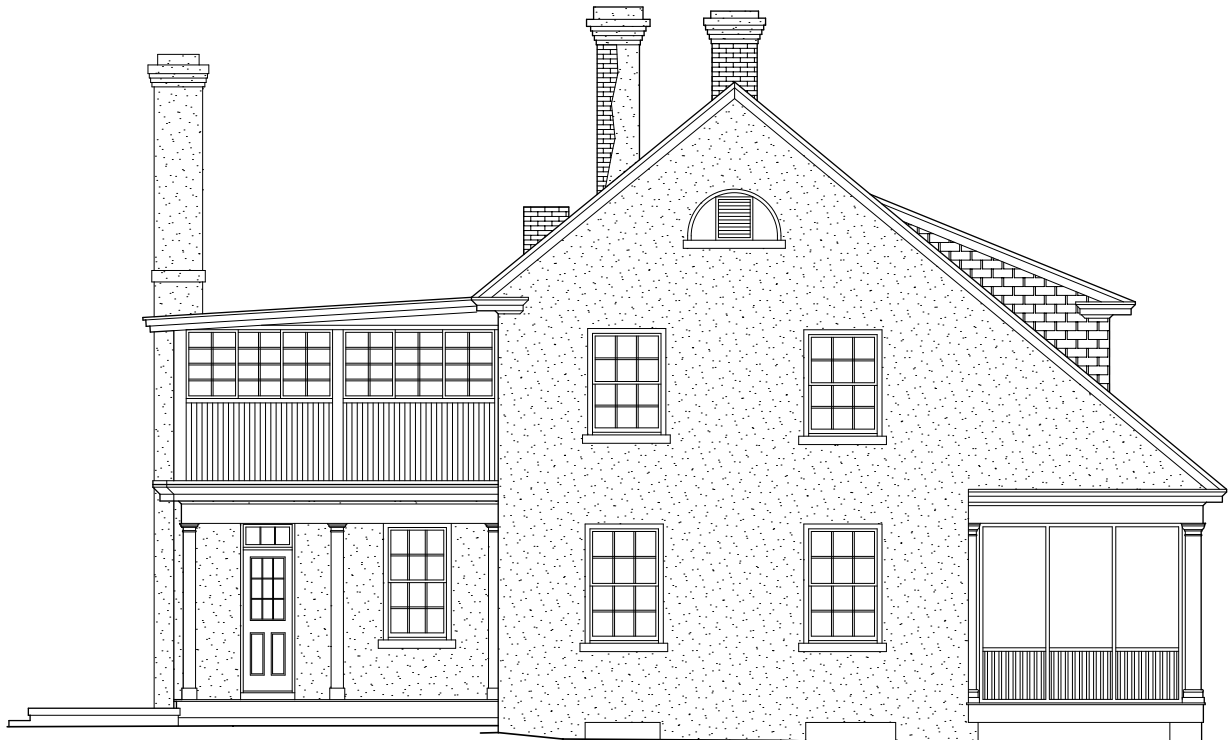
Figure 3.21 The west elevation drawing shows the rectangular vent placed in the lunette window opening.
