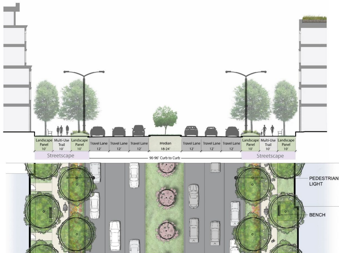
Figure 33 – Multimodal Through Corridor Cross-section
