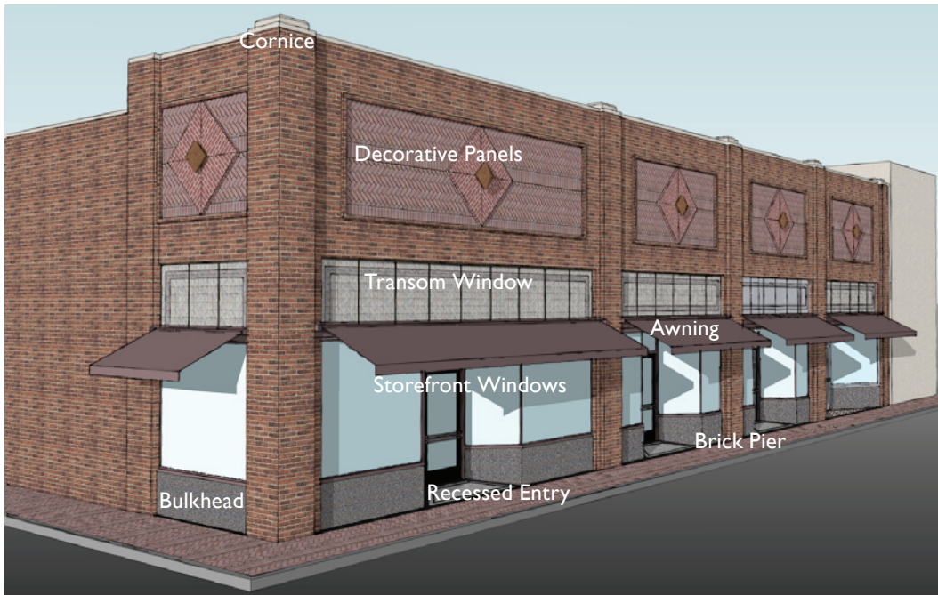
This model of an early-twentieth-century, one-story commercial building shows the typical elements of a commercial facade.
