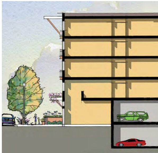
Figure 15 Example of Below Ground/Podium Structured Parking Behind Active Uses
