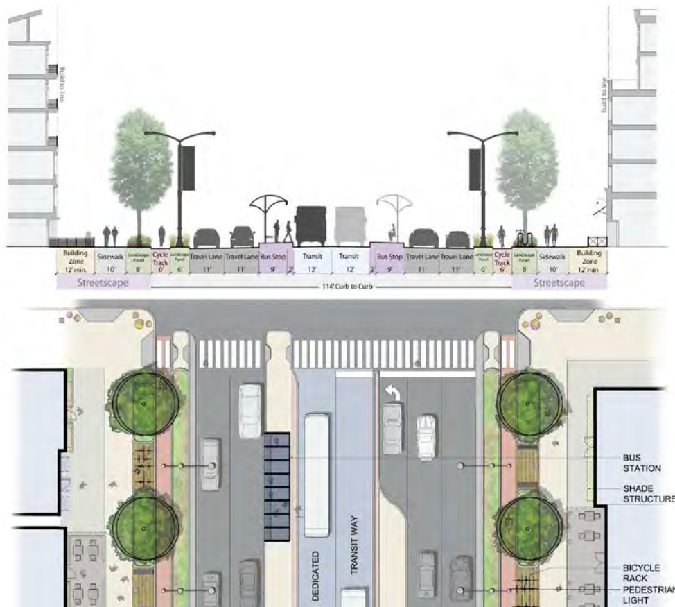
Figure 35 – Transit Boulevard Median Running Cross-section
