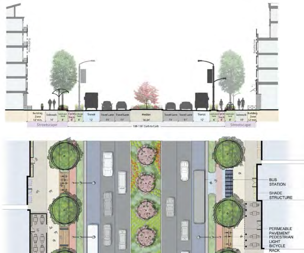
Figure 36 – Transit Boulevard Curb Running Cross-section
