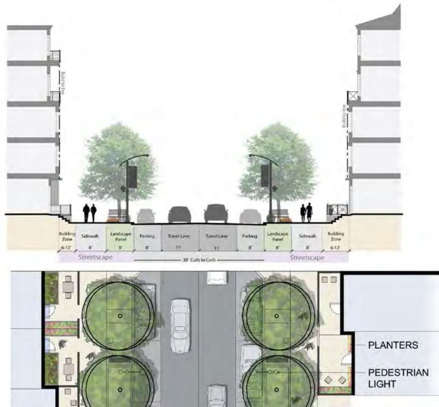
Figure 38 – Local Street Cross-section
