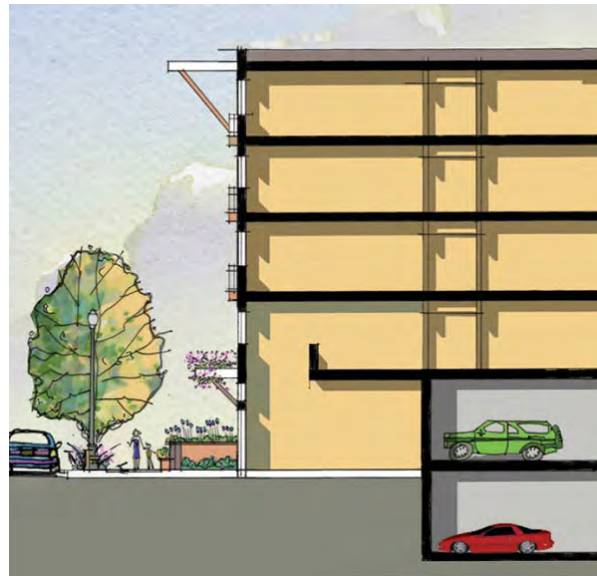
Figure 15 Example of Below Ground/Podium Parking
