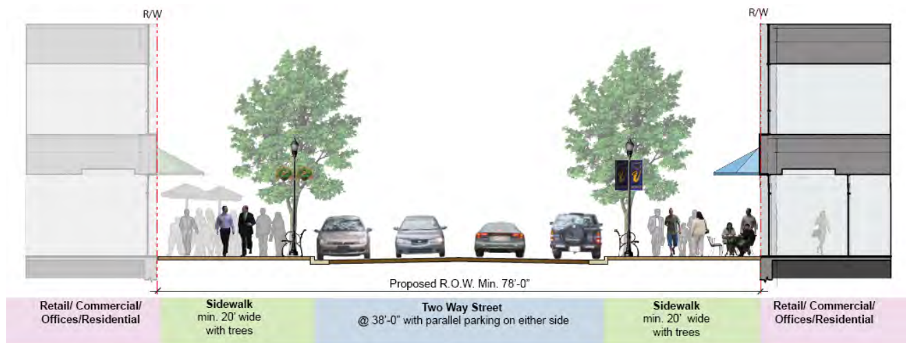
Figure 20: Typical Local Street Type 1 Cross-Section
