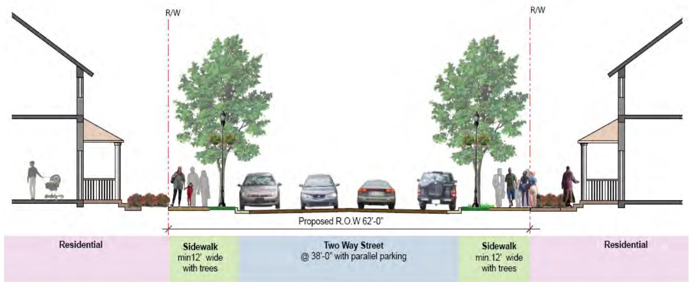
Figure 22: Typical Local Street Type 2 Cross-Section
