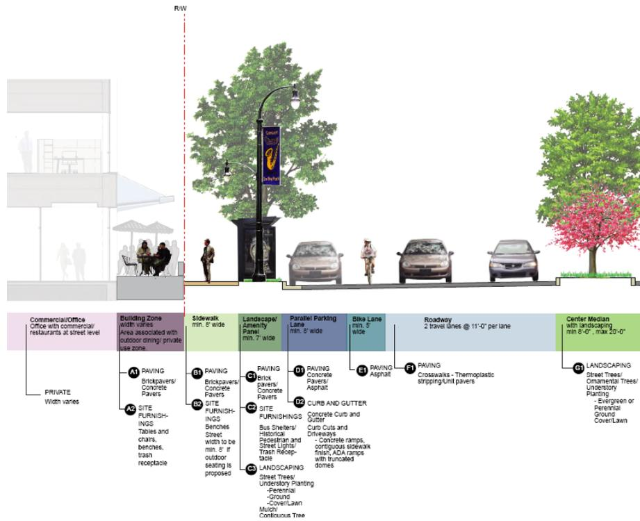
Figure 15: Minor Arterial half-section without on-street parking:
