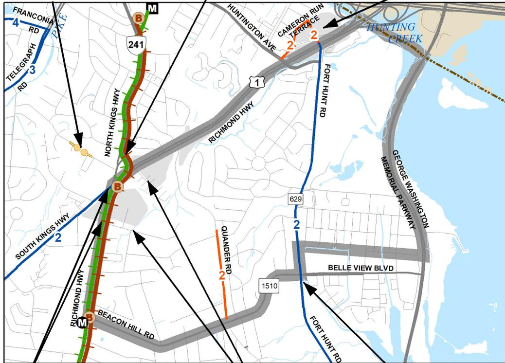
SEVER THE EXISTING CONNECTION OF SOUTH/NORTH KINGS HIGHWAY WITH RICHMOND HIGHWAY, CONCURRENT WITH THE PROVISION OF A NEW ROAD CONNECTION BETWEEN RICHMOND HIGHWAY AND SOUTH KINGS HIGHWAY IN THE GENERAL AREA, LOCATION TO BE DETERMINED WITH FUTURE STUDY
