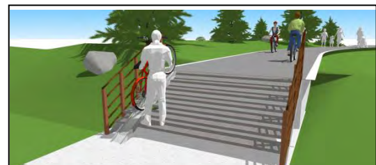
Figure 13: Rolling tray rendering Source: Toole Design Group.
