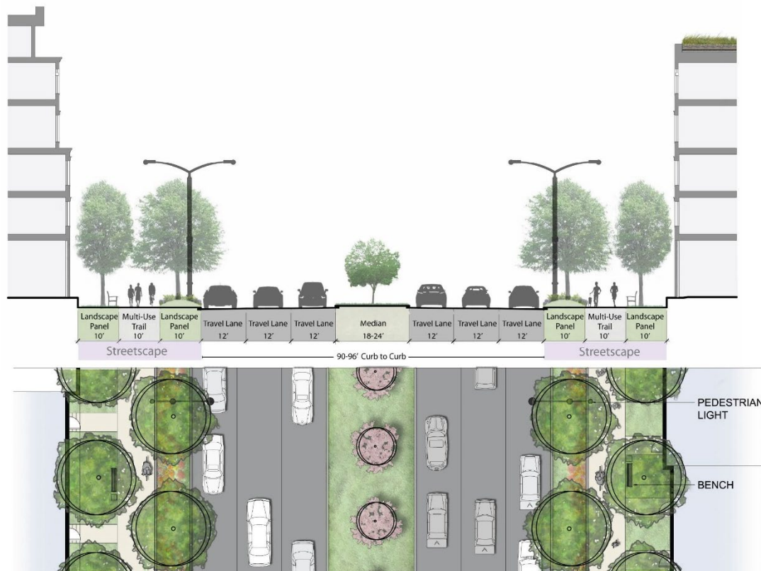
Figure 33 – Multimodal Through Corridor Cross-section
