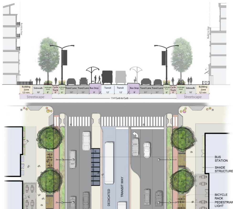
Figure 34 – Transit Boulevard Median Running Cross-section
