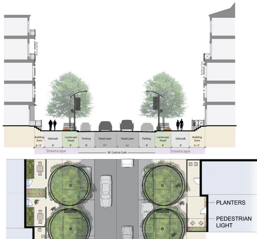
Figure 37 – Local Street Cross-section
