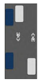
Figure 3: Shared lane marking concepts Source: Toole Design Group.
