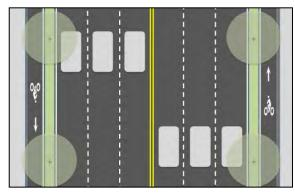
Figure 9: Cycle track concept Source: Toole Design Group.
