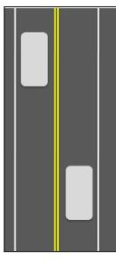
Figure 5: Striped paved shoulders concept Source: Toole Design Group.
