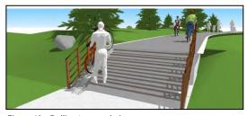
Figure 13: Rolling tray rendering Source: Toole Design Group.
