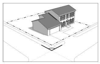
Figure 9102.2: Interior Angle of Intersection
