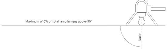
Figure 5109.1: Full Cut-Off Lighting Fixture
