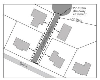
Figure 5100.11: Setback Measurement on Pipestem Lots
