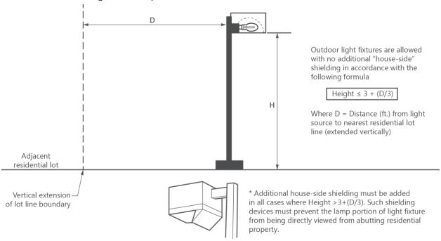
Figure 5109.4: Mounting Height or House-Side Shielding
