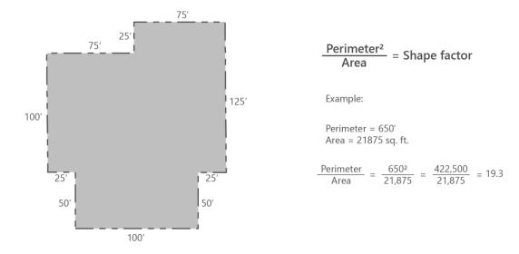
Figure 5100.10: Shape Factor Calculation
