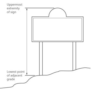
Figure 7100.5: Measuring Height of Freestanding Signs
