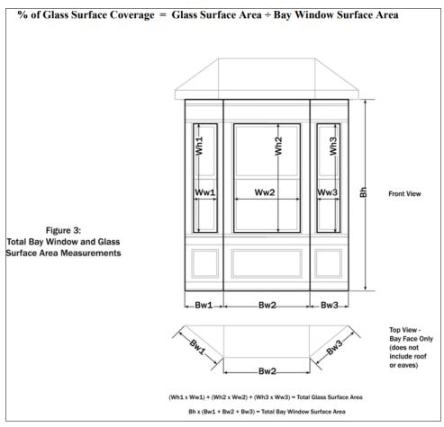
Figure 5100.3: Bay Window Glass Surface Coverage
