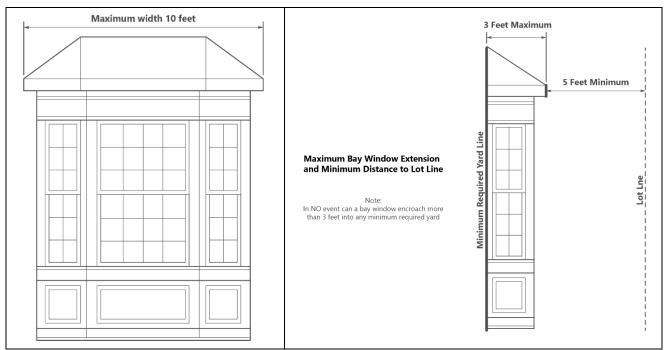
Figure 5100.2: Bay Window Extension into Required Setback
