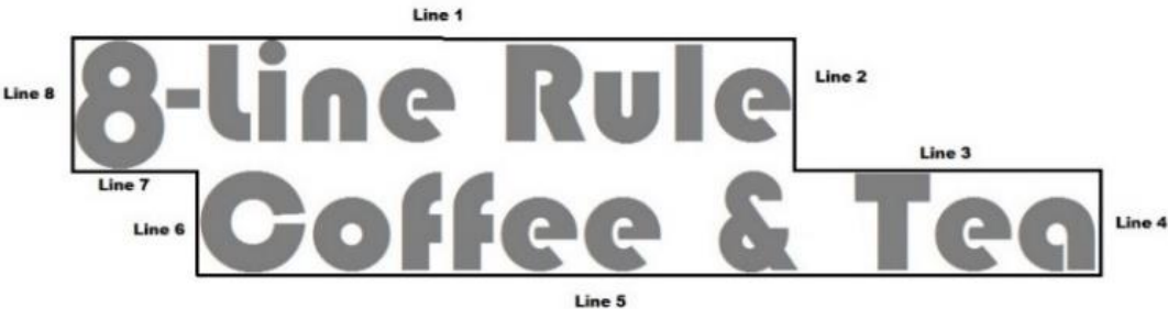
Figure 7100.2: Measuring Building-Mounted Sign Area
