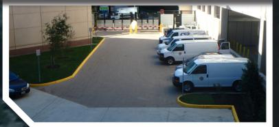
The PSHQ service driveway is paved with permeable pavers. These interlocking brick pavers allow water to drain through the gaps between the bricks into a gravel base below. The water then infiltrates or slow flows into the storm drain system that discharges to the wet pond.
