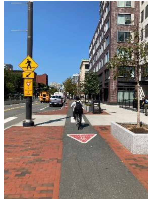
Off-Street One-Way Cycletrack
