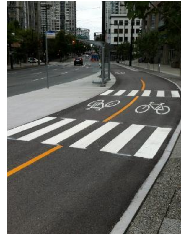
Off-Street Two-Way Cycletrack
