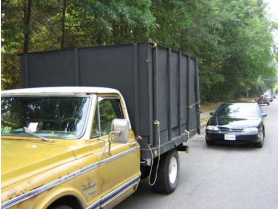
Less than 8 feet high, less than 21 feet long, 4000 lbs GVW per DMV
