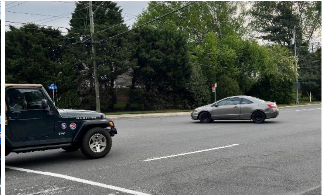
Vehicle turning left from Platten Drive onto westbound Blake Lane conflicts with vehicle turning left from Blake Lane onto Edgelea Road
