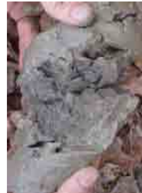
Figure 5: Completely gleyed, low-chroma soil matrix.
