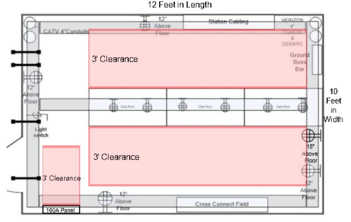
Figure 1 Telecommunications Room Electrical Requirements
