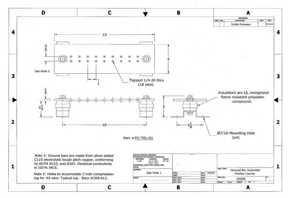
Figure 2. Telecommunications Room Grounding Requirements
