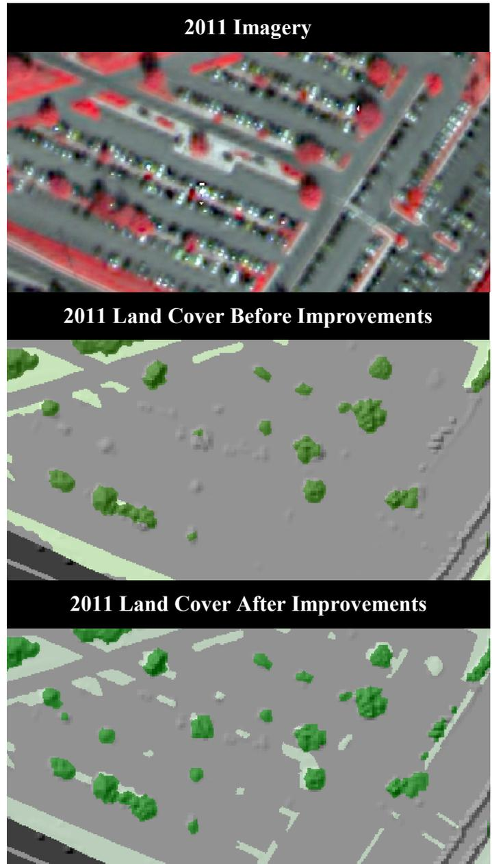
Figure 4: Small Trees that were omitted from the 2011 land cover dataset were picked up in the improved 2011 dataset by using the Tree Canopy classification from the 2015 land cover assessment. The comparison of the Normalized Digital Surface Model (height above ground) between the two LiDAR datasets proved to be a valuable method in detecting these small trees.
