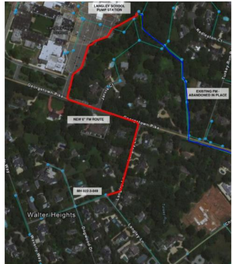
The red line shows the proposed force main. The blue line shows the existing force main that will be abandoned-in-place.
