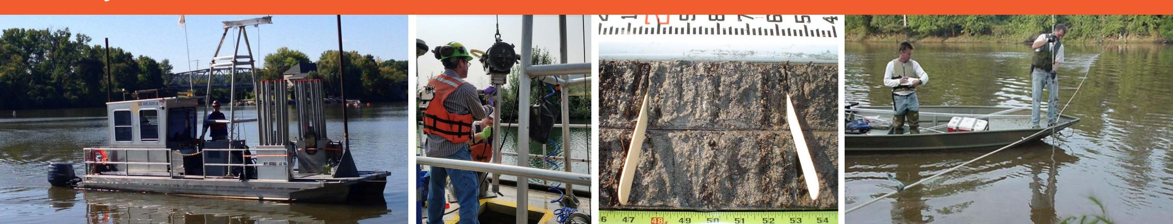
Sampling teams will move around Lake Accotink using a Vibracore pontoon boat As shown in the picture to the right, a sampling tube is lowered to the sediment surface and then the Vibracore head vibrates the tube advancing it through the sediment to collect an undisturbed sample core from the lake sediments.
