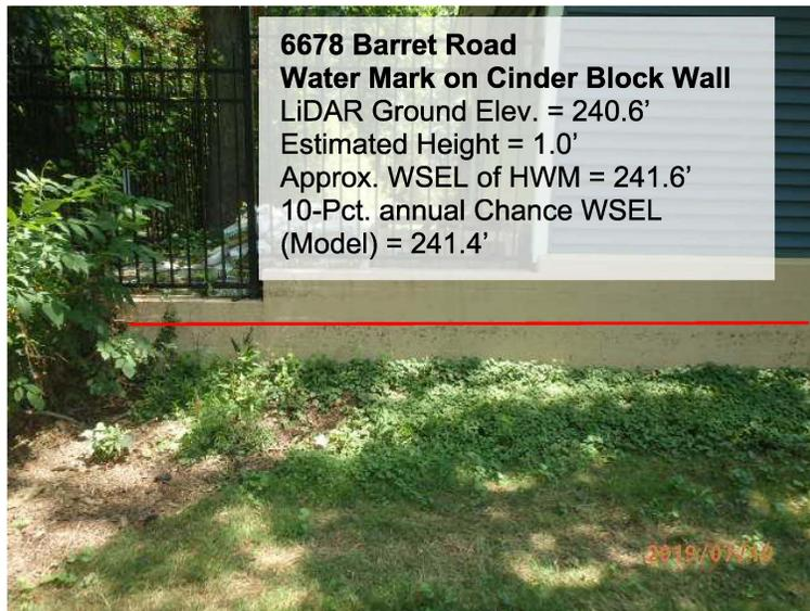
Figure 5 -- Example of an Approximate High Water Mark (HWM)
