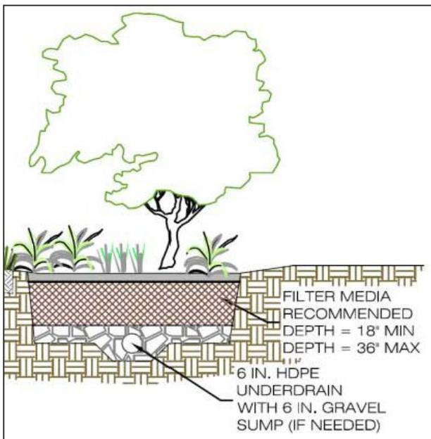
Figure 4-5: Bioretention section
