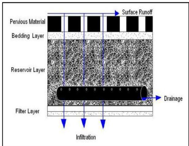
Figure 4-6: Pervious pavement section
