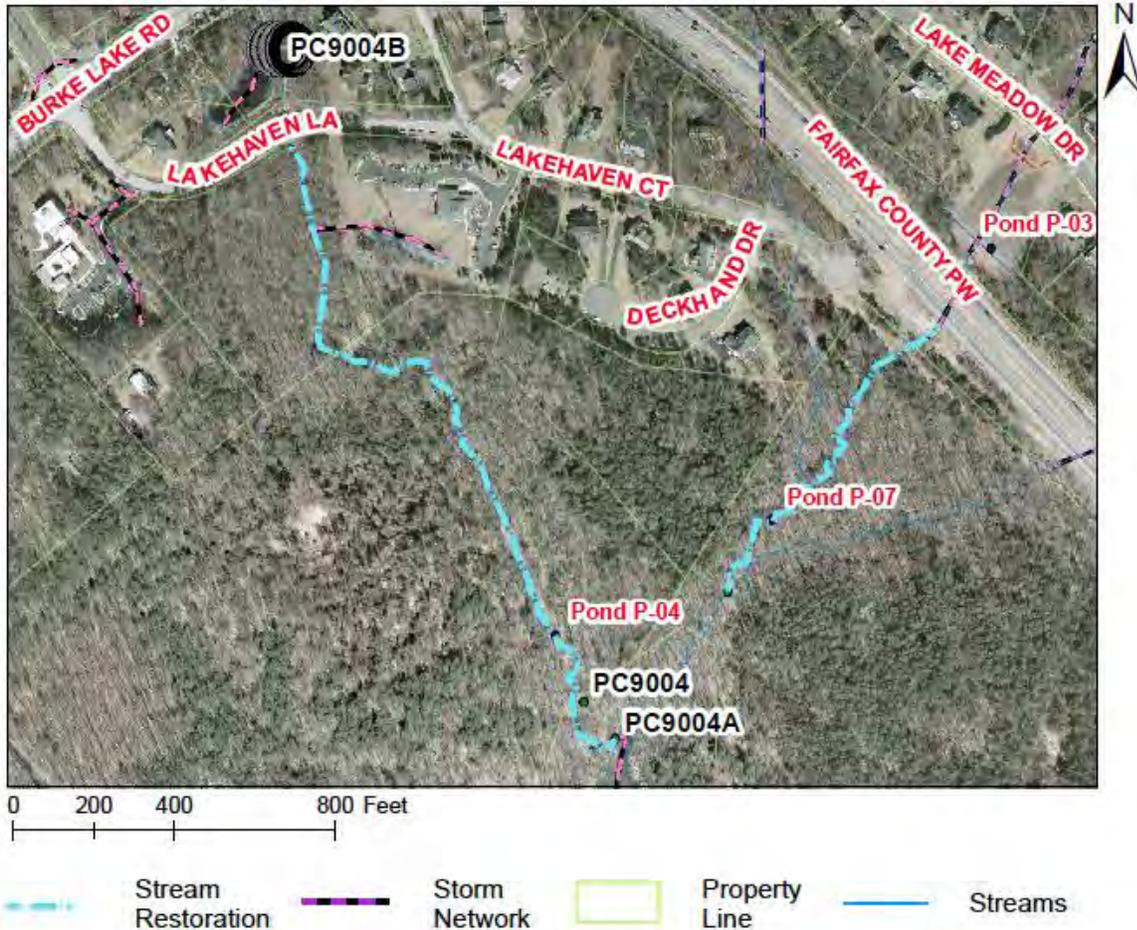
**Project Benefits:** The stream stabilization will reduce sediment loads to the stream, maintaining the capacity of the stream and controlling unwanted meander. Removing the obstruction will help restore the stream channel to its natural conditions and improve the function of the stream. This suite of projects will help to return the stream to its natural condition and reduce pollutant loads and erosion. Below are the project's estimated pollutant removal amounts.
