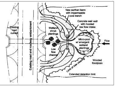
Figure 4.2: Culvert Retrofit
