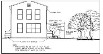
Figure 4.8: Rain barrel
