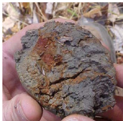
Figure 3: Iron oxidized mottling of a gleyed soil matrix.
