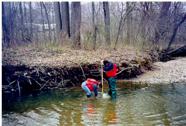
Benthic macroinvertebrate samples are collected from riffles and shallow runs, the most productive areas in streams.
