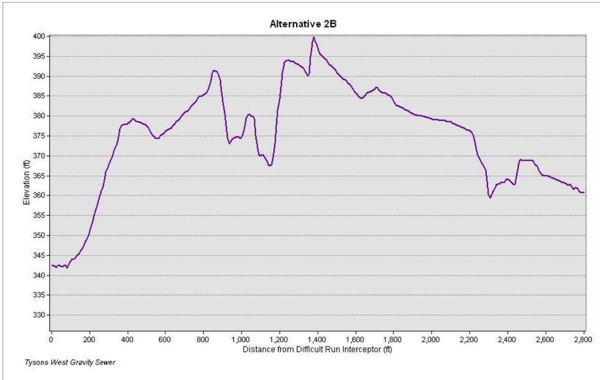
Figure-5: Grade elevation for Alternative-2B route
