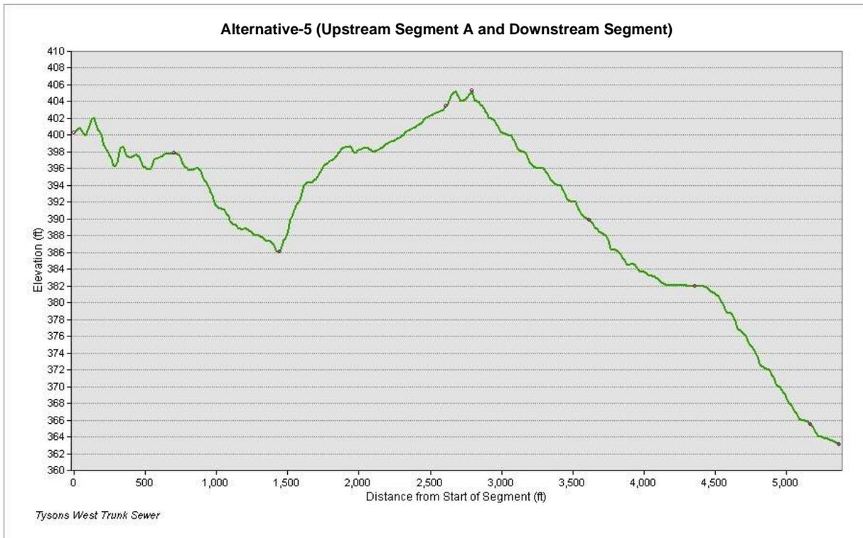
Figure-11: Grade elevation for Alternative-5 route
