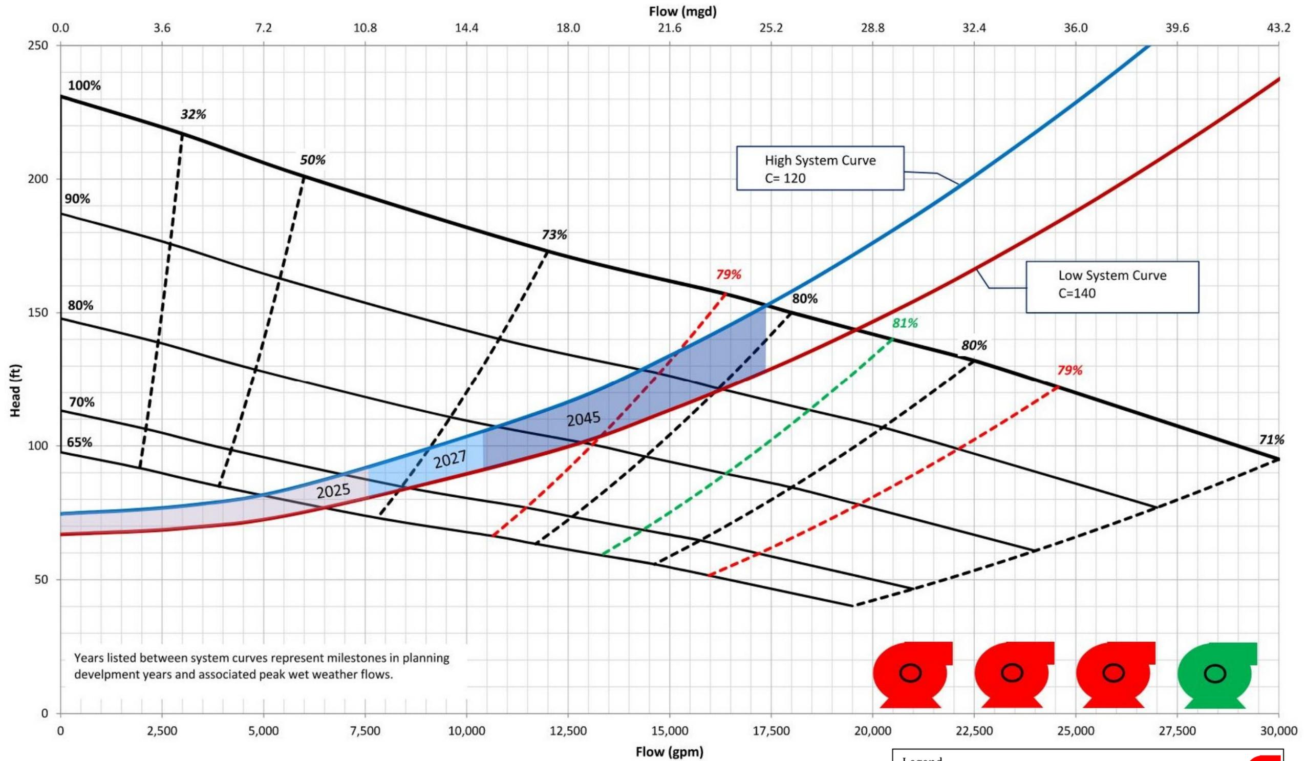
Figure 3-11: Preliminary pump and system curves with three pumps in operation.
