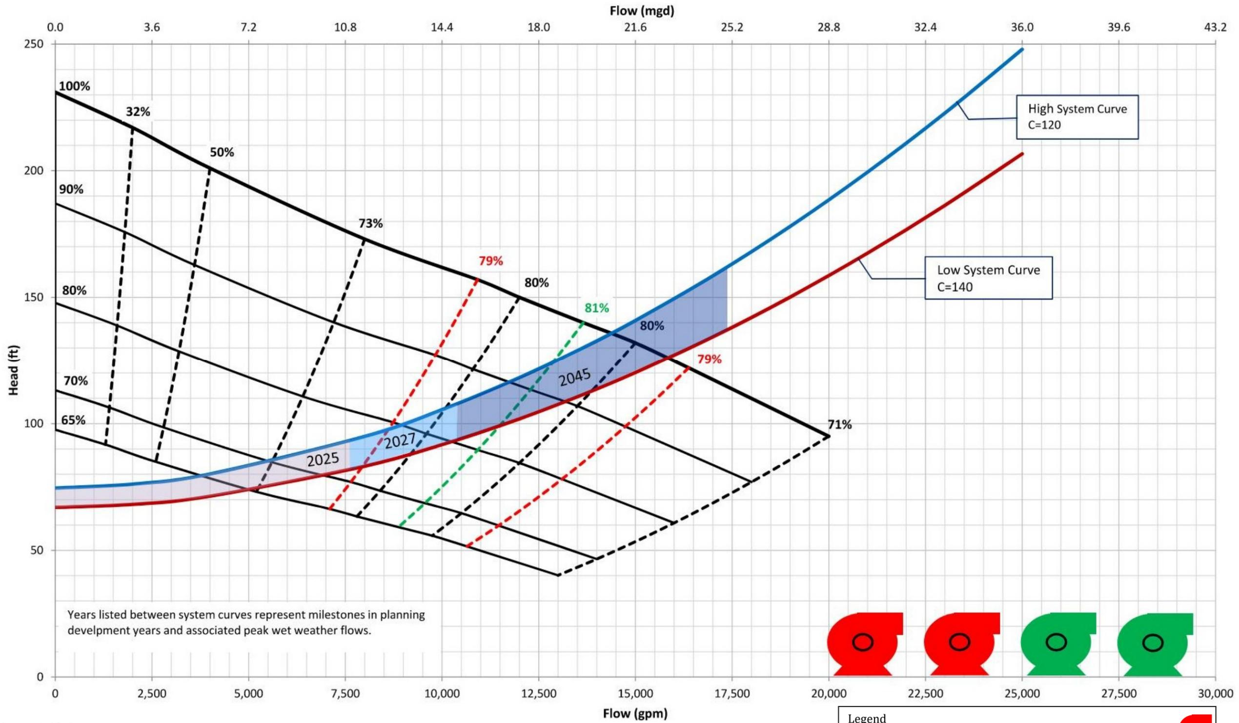
Figure 3-10: Preliminary pump and system curves with two pumps in operation.
