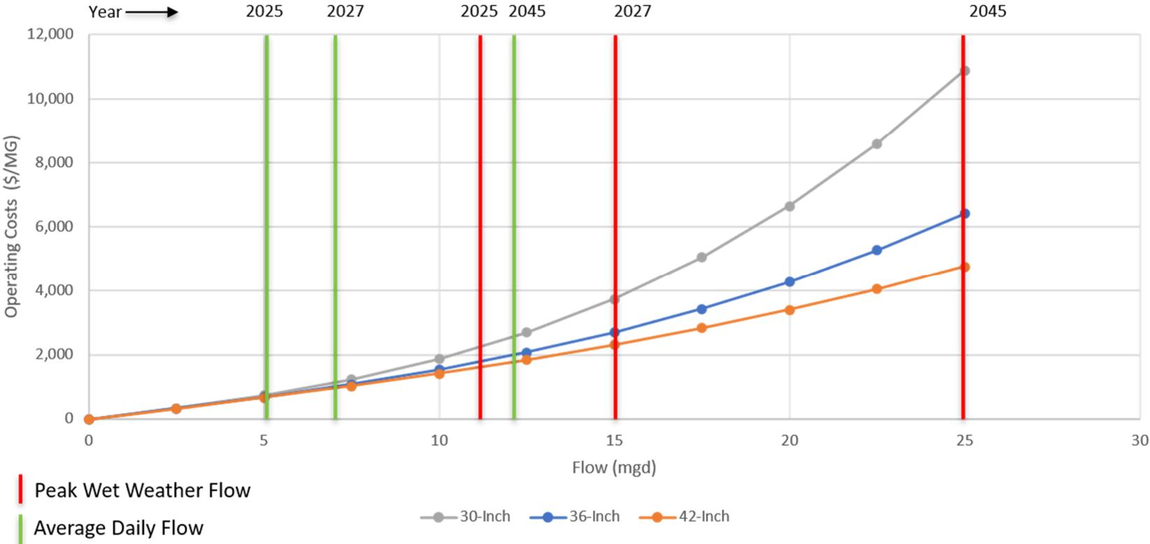
Figure 3-8: Operating costs profile for three different force main diameter alternatives.
