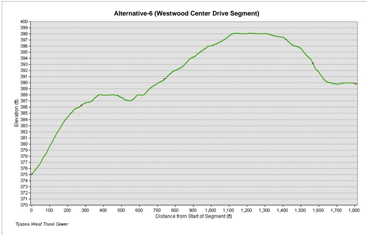
Figure-16: Grade elevation for Alternative-6 route Westwood Center Drive Segment
