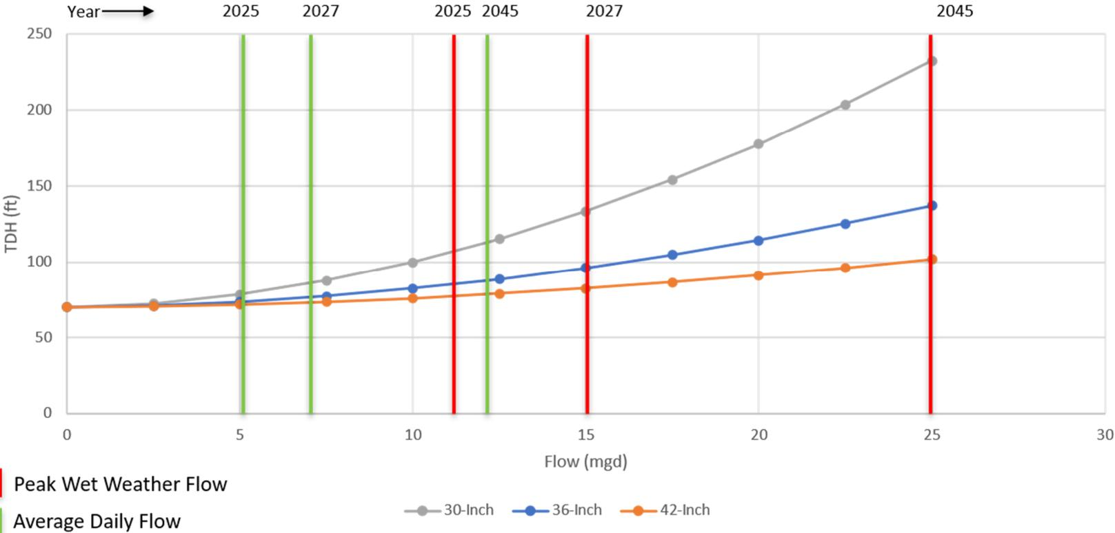
Figure 3-6: Total dynamic head profile for three different force main diameter alternatives.
