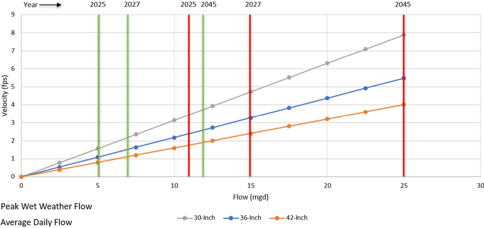
Figure 3-4: Velocity profile for three different force main diameter alternatives.
