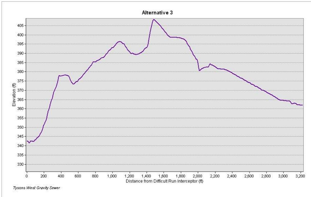
Figure-7: Grade elevation for Alternative-3 route
