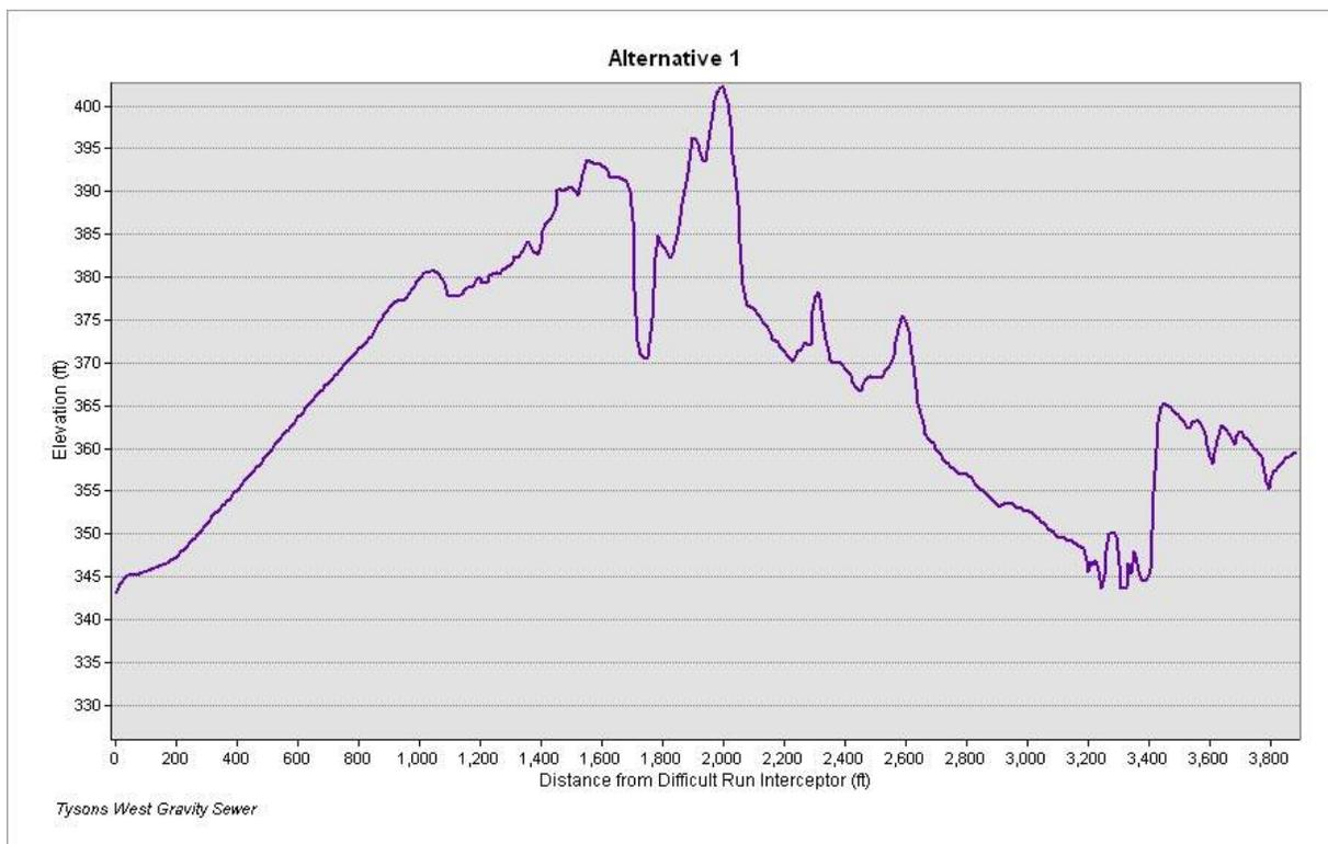
Figure-2: Grade elevation for Alternative-1 route
