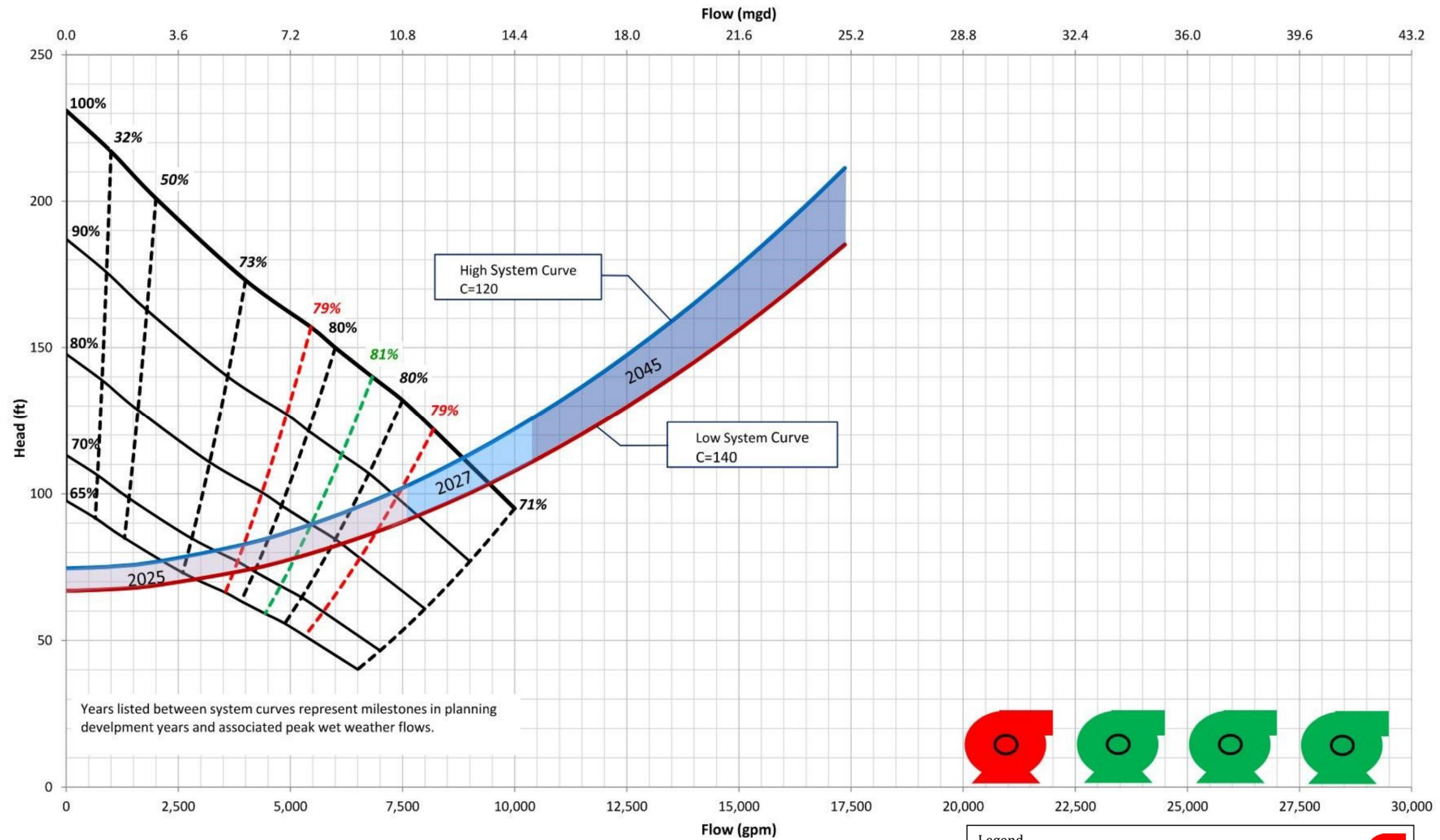
Figure 3-9: Preliminary pump and system curves with one pump in operation.
