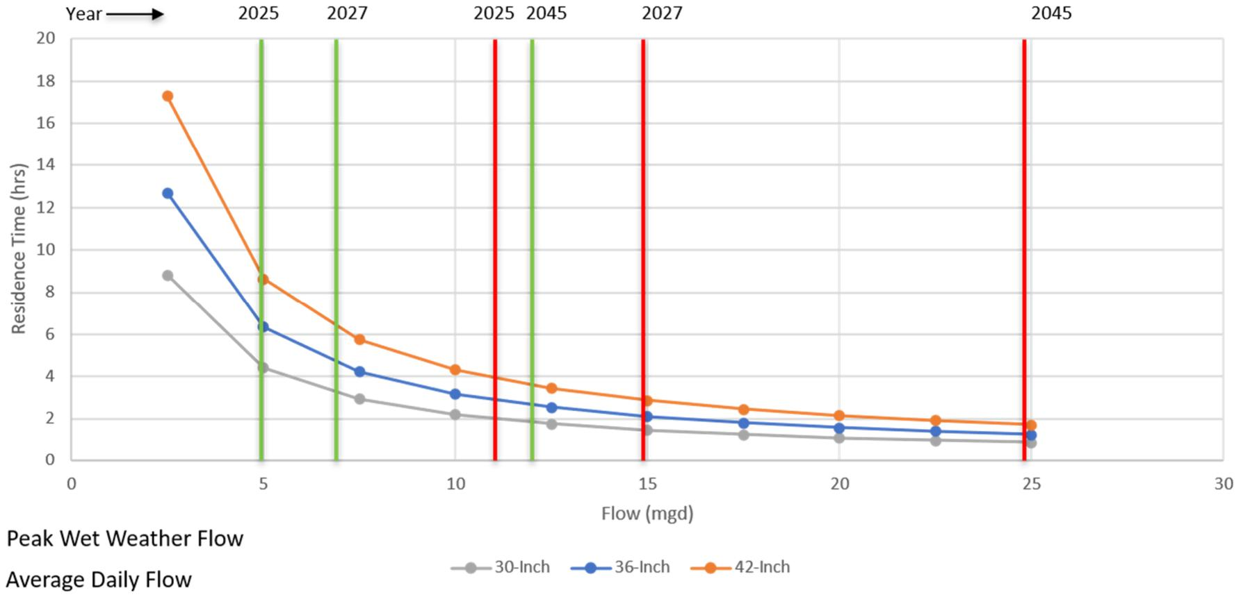
Figure 3-5: Residence time profile for three different force main diameter alternatives.
