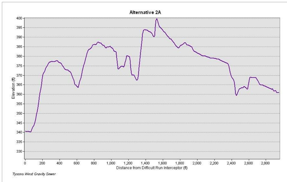
Figure-4: Grade elevation for Alternative-2A route
