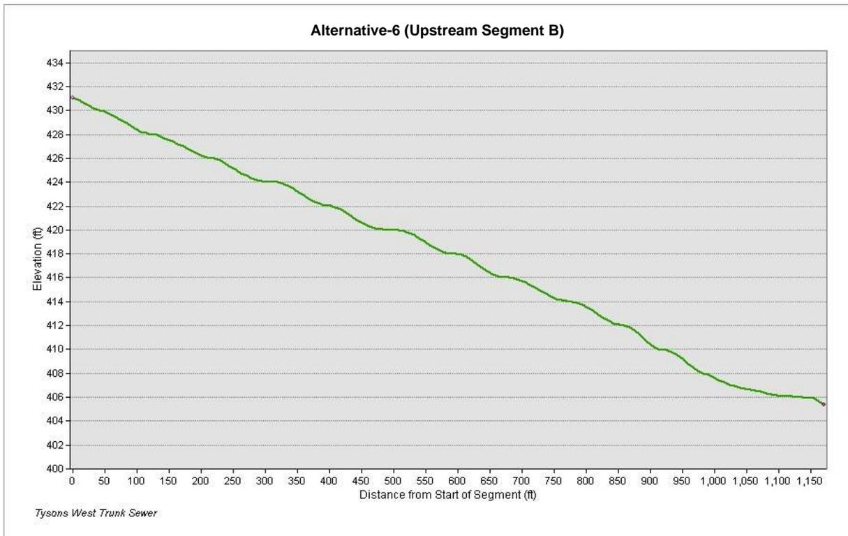
Figure-15: Grade elevation for Alternative-6 route Upstream Segment B
