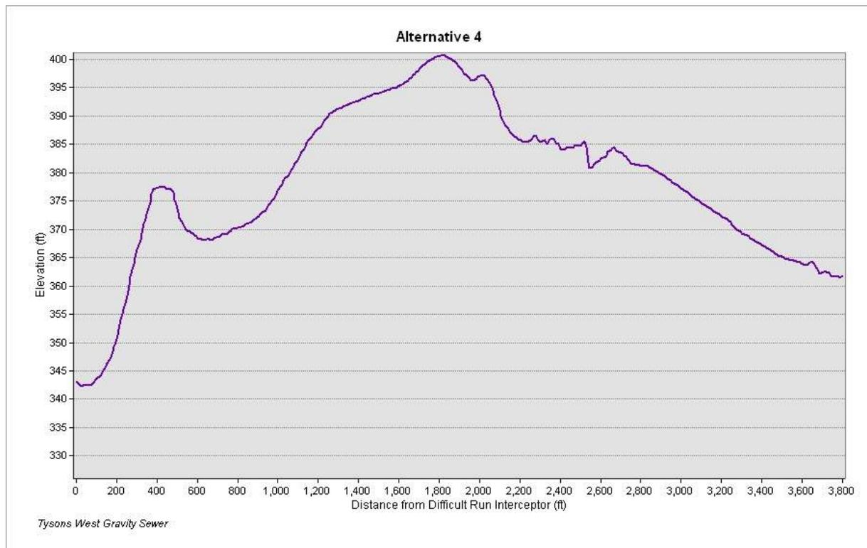
Figure-9: Grade elevation for Alternative-4 route
