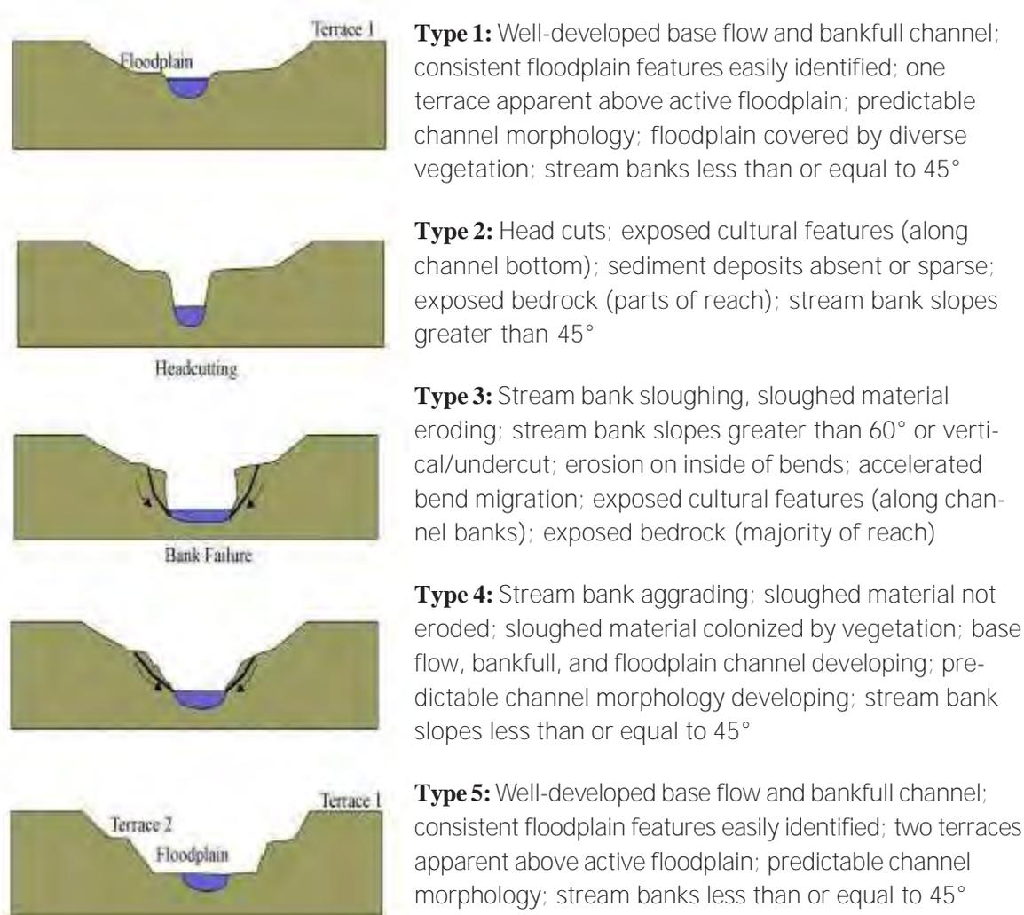
Figure 2.4 Incised Channel Evolution Model (Schumm, Harvey, and Watson, 1984)
