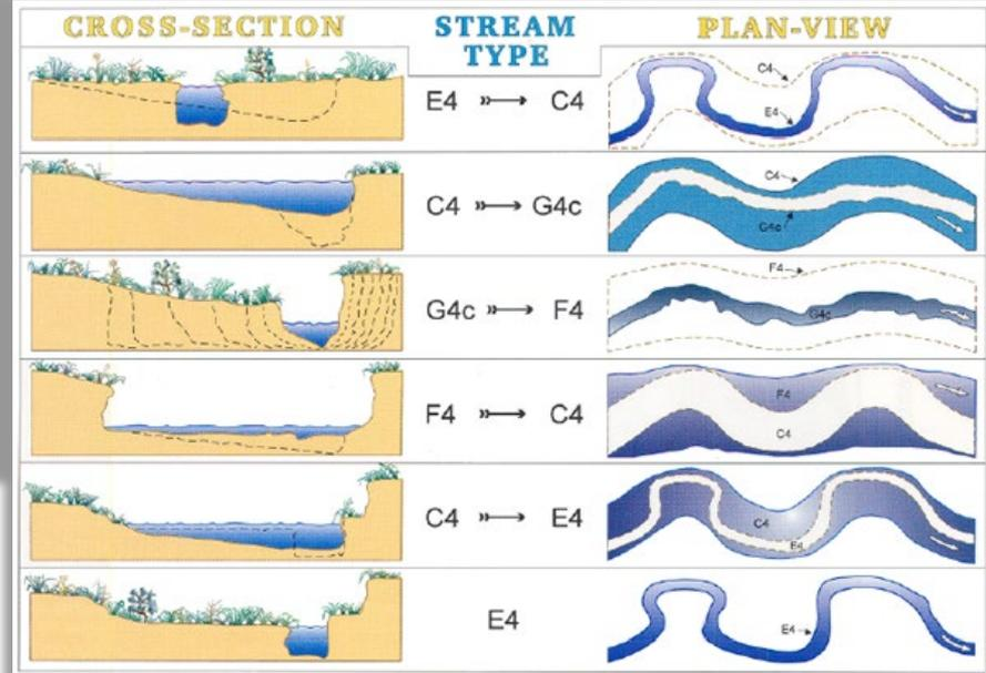
Adjustments of channel cross-section and plan-view patterns as stream types change or shift through an evolutionary cycle (Rosgen 1996)
