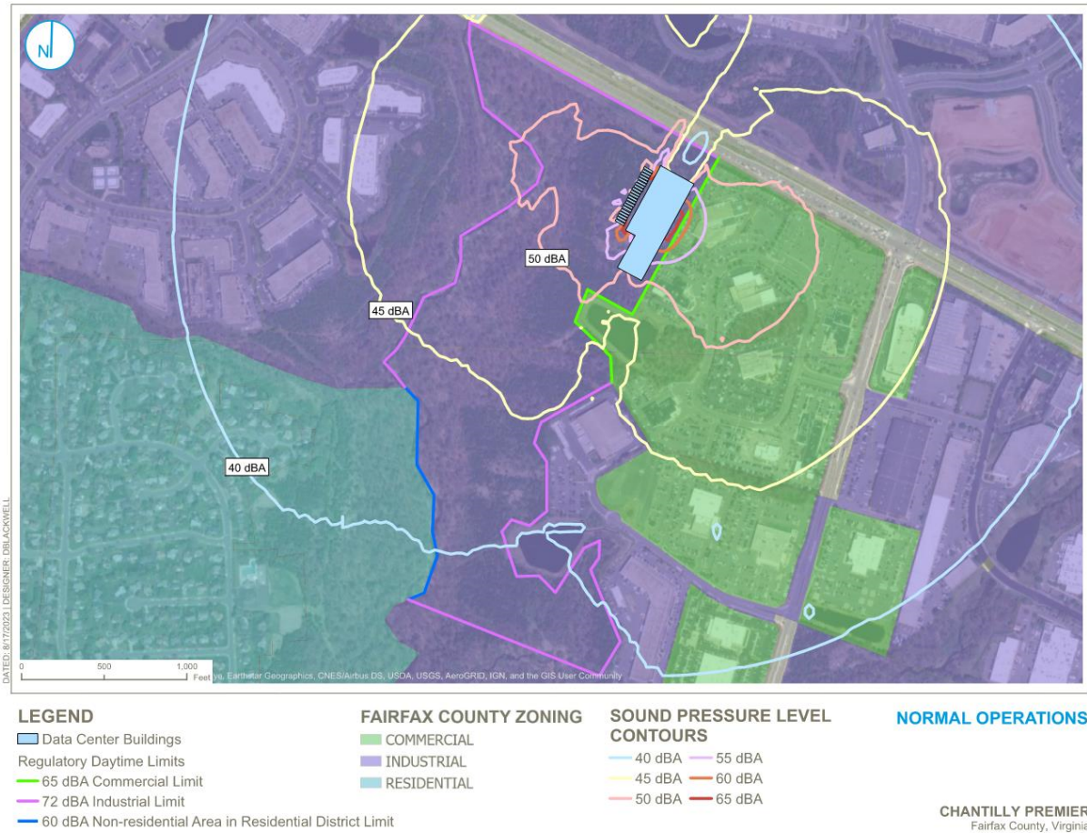
Figure 1 - Project sound emissions full load daytime operation
