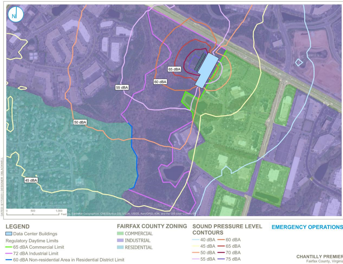
Figure 3 - Project sound emissions during emergency operations and simultaneous testing of all generators
