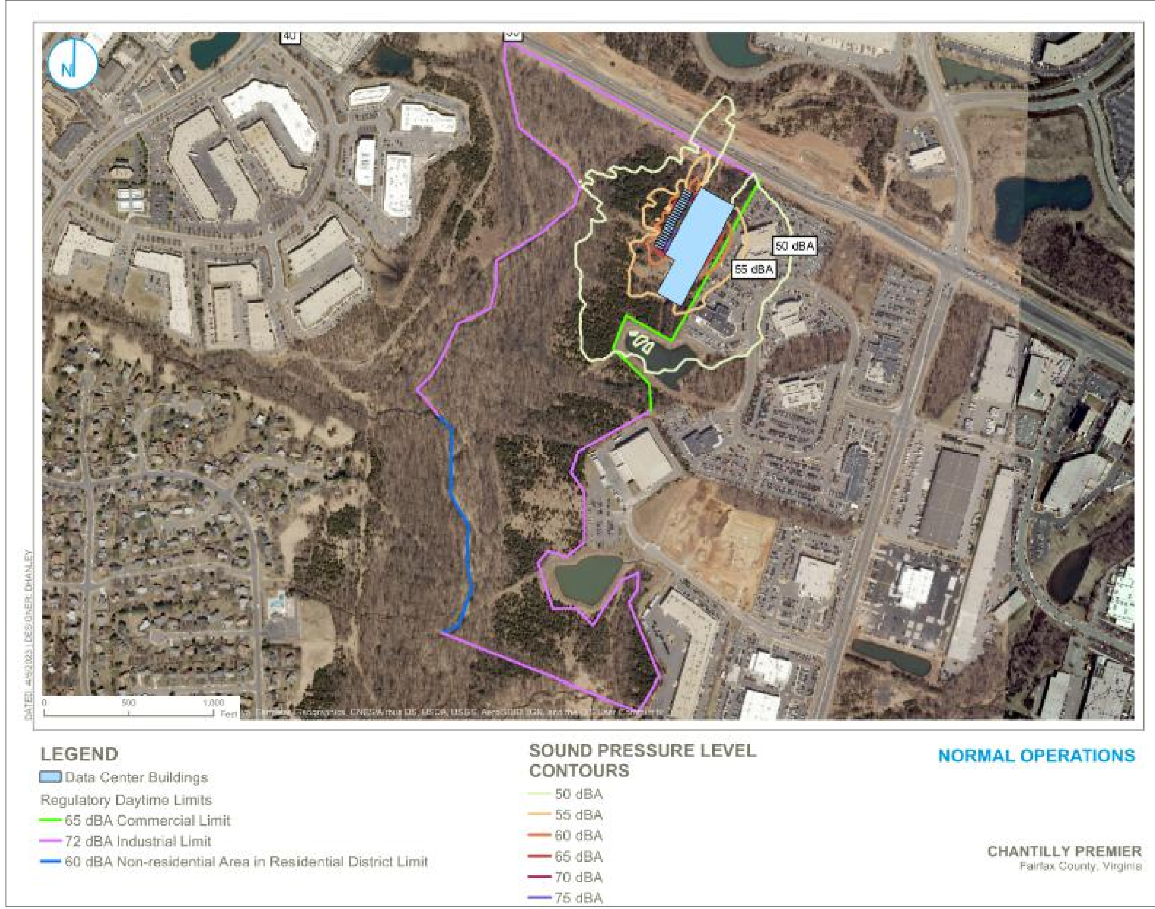
A PROJECT SOUND EMISSIONS DURING NORMAL DAYTIME OPERATION N.T.S.
