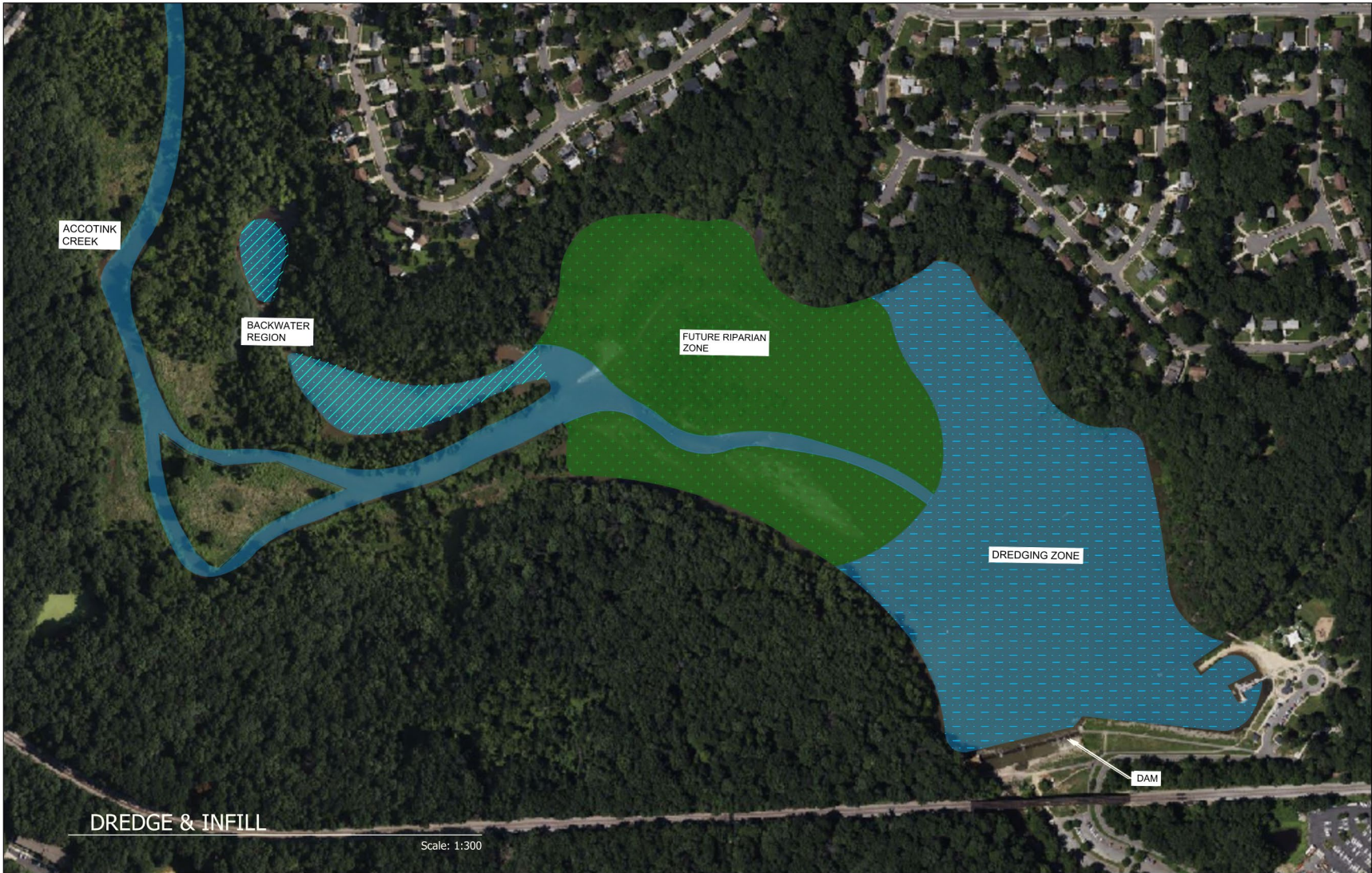
Figure 3-6. Partial dredge with dam modification scenario
