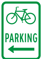
Sign D4-3, Manual on Uniform Traffic Control Devices for Streets and Highways (MUTCD)
