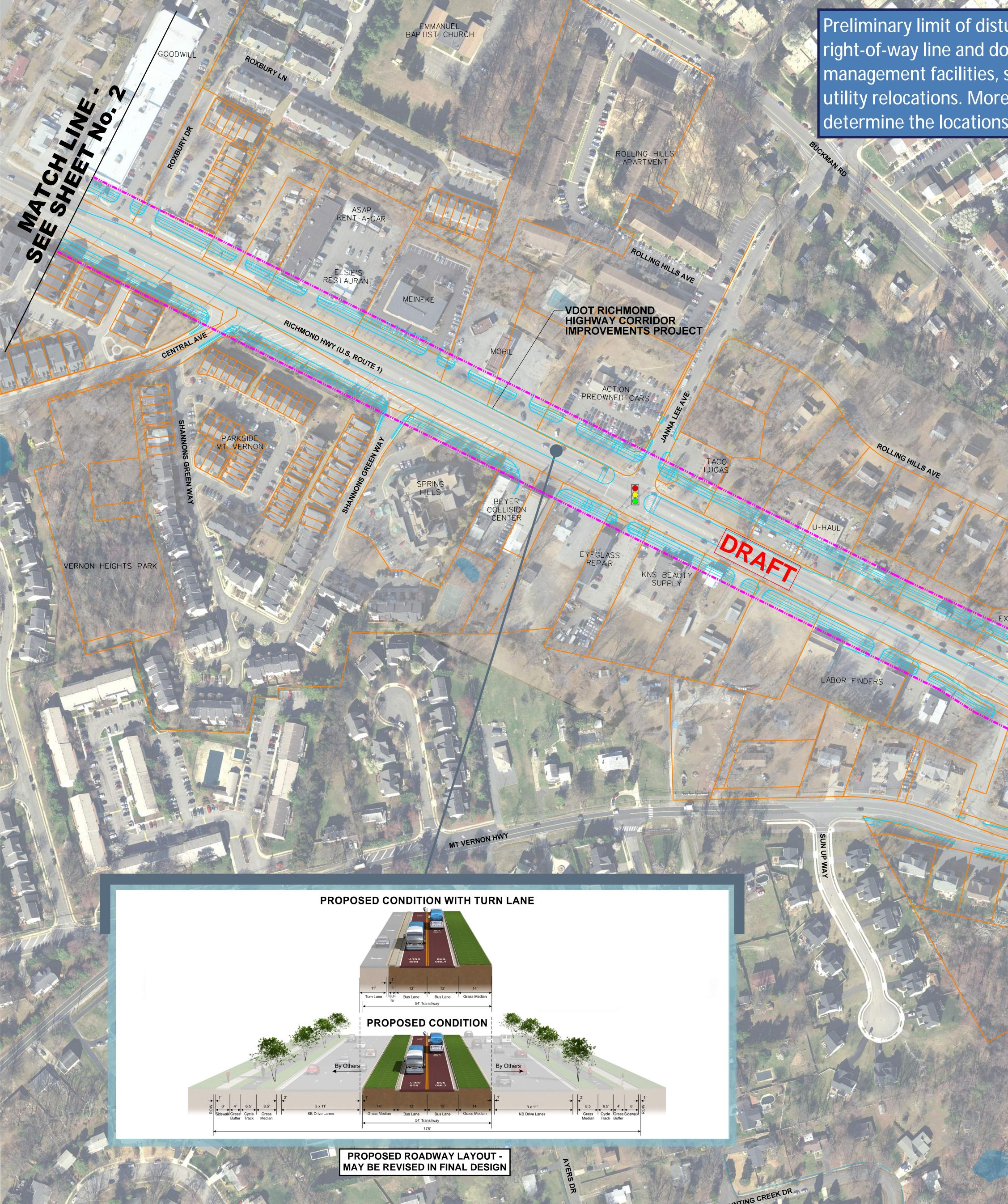
Preliminary limit of disturbance does not represent a right-of-way line and does not include stormwater management facilities, side street improvements, or ility relocations. More detailed analysis is required to determine the locations and impacts of these features.
