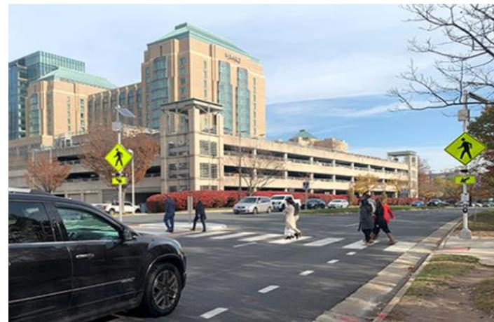
Rectangular Rapid Flash Beacon (RRFB) are bright flashing lights that are activated by pushing a button. The lights warn drivers that a person is crossing the road. Pedestrians still have to wait for a safe gap in traffic before crossing.
