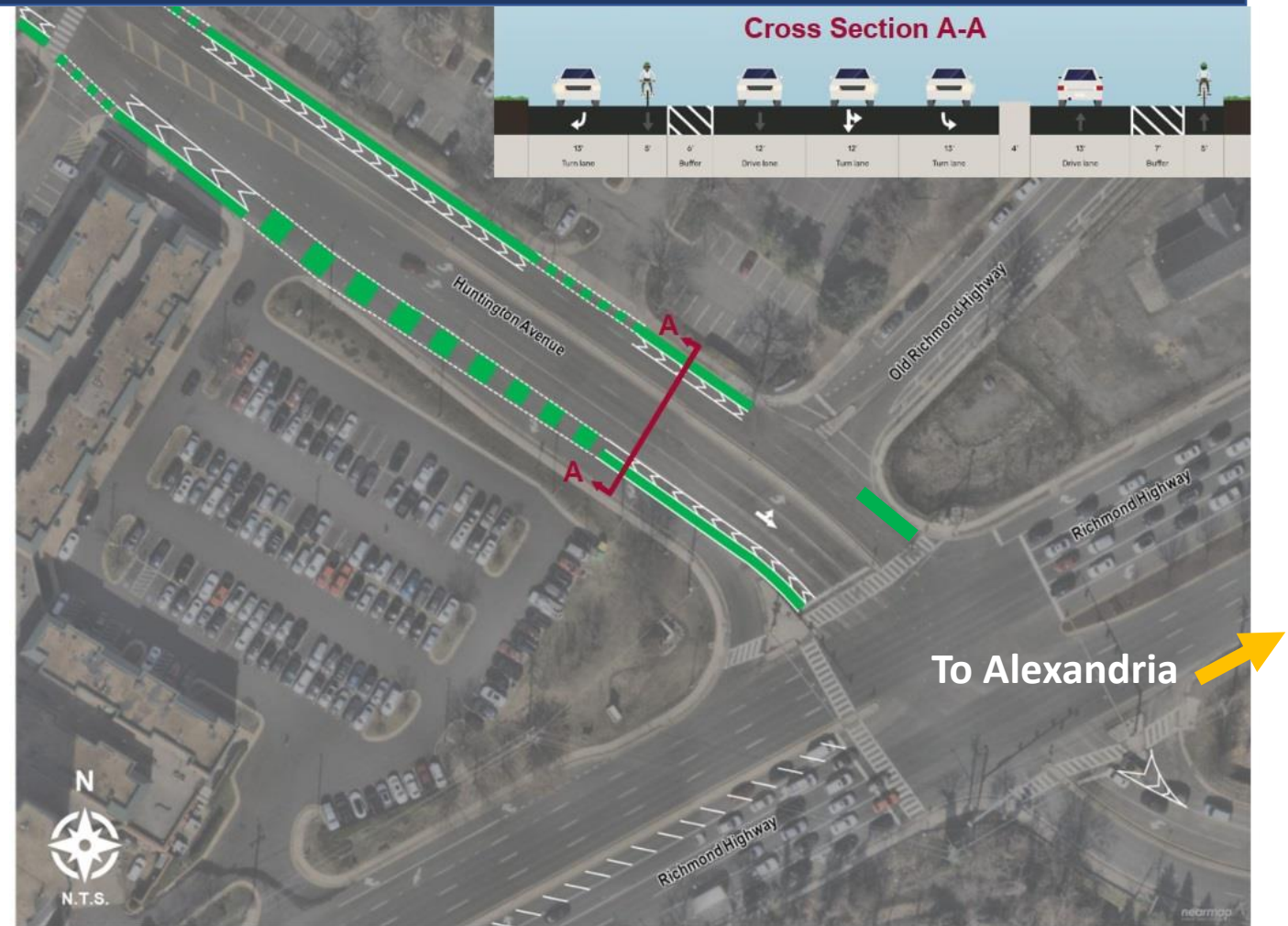
Figure 11: Intersection of Huntington Avenue and Richmond Highway Build Conditions Cross Section and Plan View
