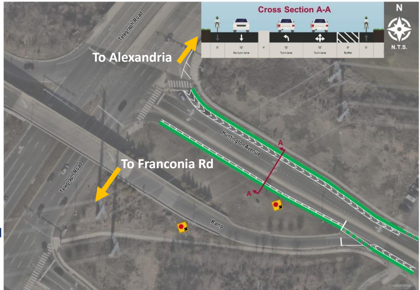
Figure 10: Huntington Avenue and Telegraph Road Alternative Build Conditions Cross Section and Plan View
