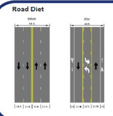
A road diet eliminates one or two travel lanes in order to provide a bicycle lane, or a buffered bicycle lane, within the existing width of the road. Typically, a center turn lane is provided for left-turn movements. In many situations, the resulting three-lane cross section functions more efficiently for motor vehicle traffic (and with fewer crashes) as well as allowing for bicycle lanes.
