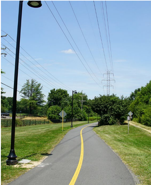
Multi-Use Hard Surface Trail Designed for Fast Travel Speeds (State Design Standards)
