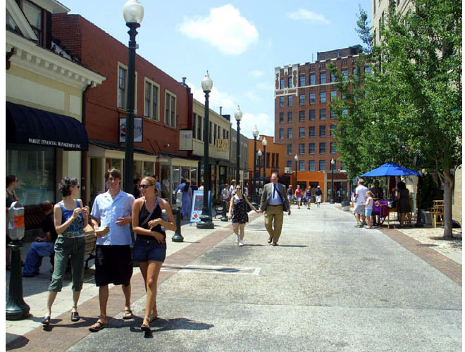
Wall Street in Asheville NC, displays a Woonerf in action. Flushed curbs, with no raised sidewalks, increases walkability. The added bollards ensure safety is not lost in this curb transition. Photo: Alyson West, PBIC Image Library.
