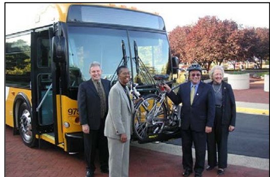
In 2007, all Fairfax Connector Buses were equipped with front mount bike racks
