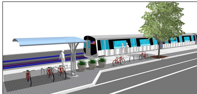
Figure 15: Rendering of covered bicycle parking at a transit station Source: Toole Design Group.
