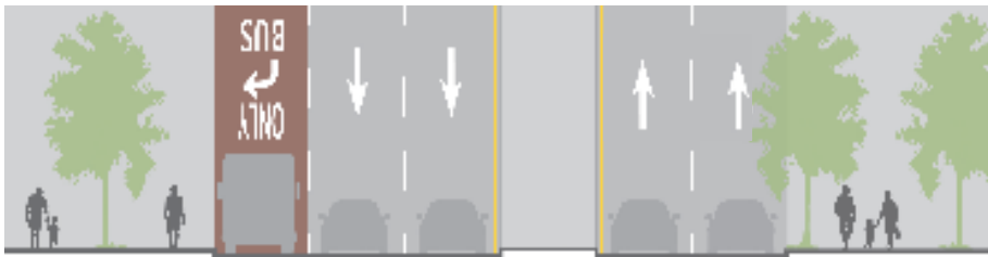
Figure 6-26 | Alternative 6 Cross-section of Chain Bridge Road from Boone Boulevard to Route 7
