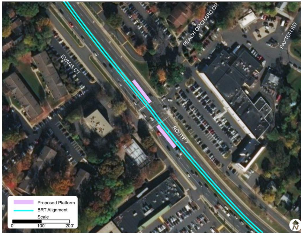
Figure 8-12 | Patterson Road Station Location and Platform Configuration
