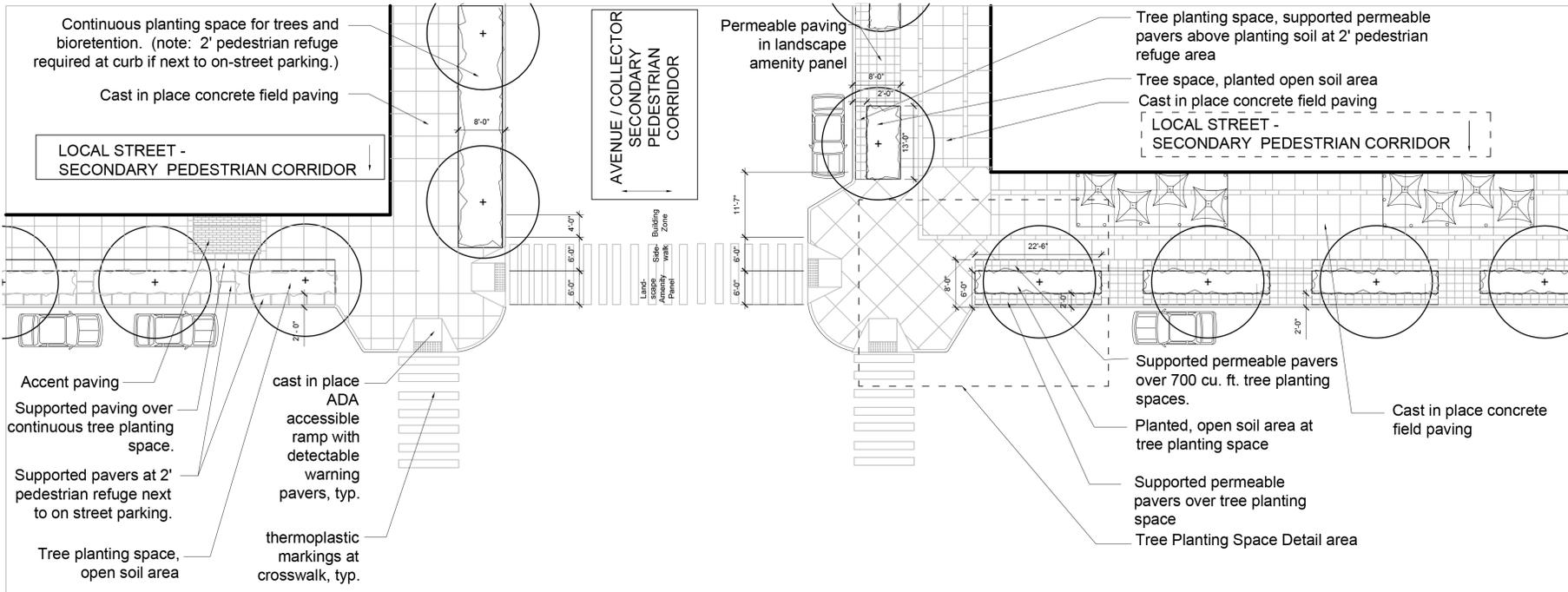
Secondary Pedestrian Corridor Paving Example - Plan
